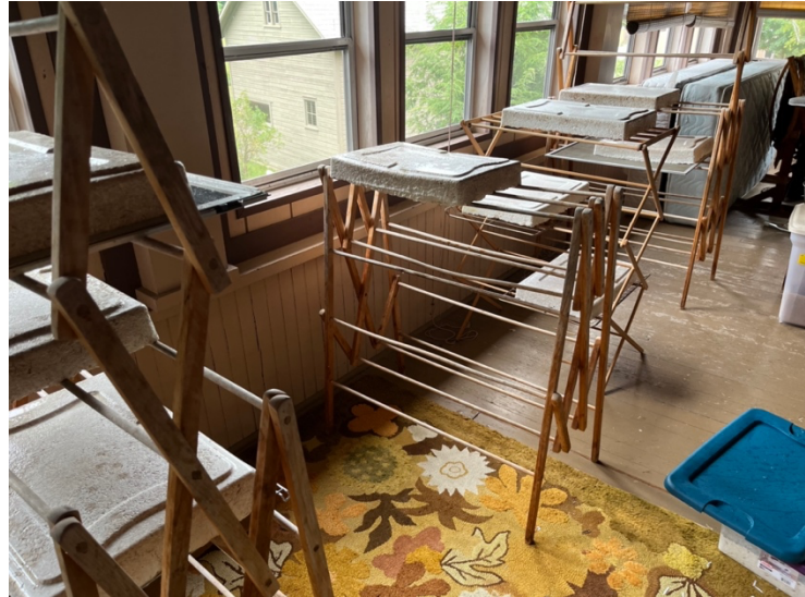
Here we see the mycelium pads, laid out on drying racks at Sue Vanhook's studio space. They were created with a custom mold to fit the cedar crates. We're very excited to add this element to our design.
